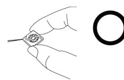
Don't pull fan with lead wires.
